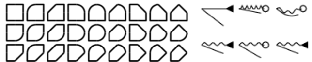
Fig 20. The four separate attributes defining the shapes on left (i.e. corners) are not as easily distinguishable as the four separate attributes defining the shapes on the right.
