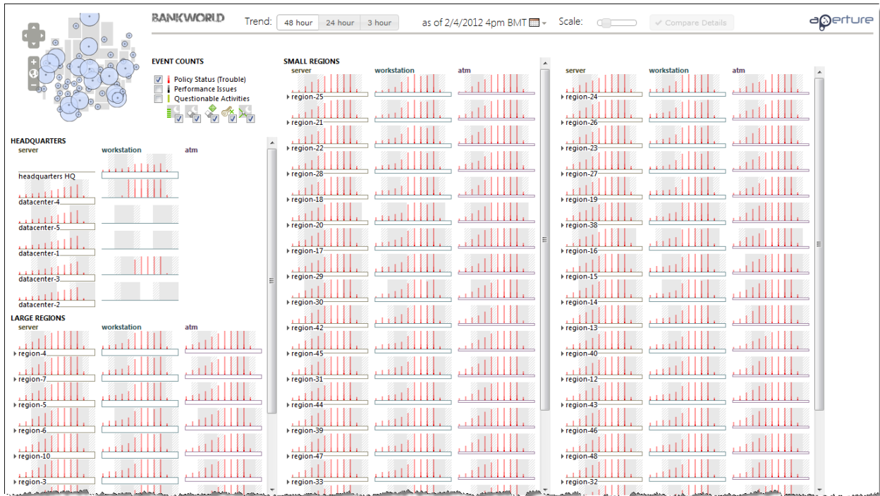
Figure 14: Cyber-situation awareness application for “BankWorld”. Using the legend to filter on policy event type we observe an upward trend in policy violations across all regions in the enterprise. The charts are generated based on normalized counts of events as a percentage of the total number of machines in the region, with the base of each time scale proportional to the number of machines. Regions are sorted by time zone, and shaded areas in each thumbnail indicate periods outside of business hours for that area.
